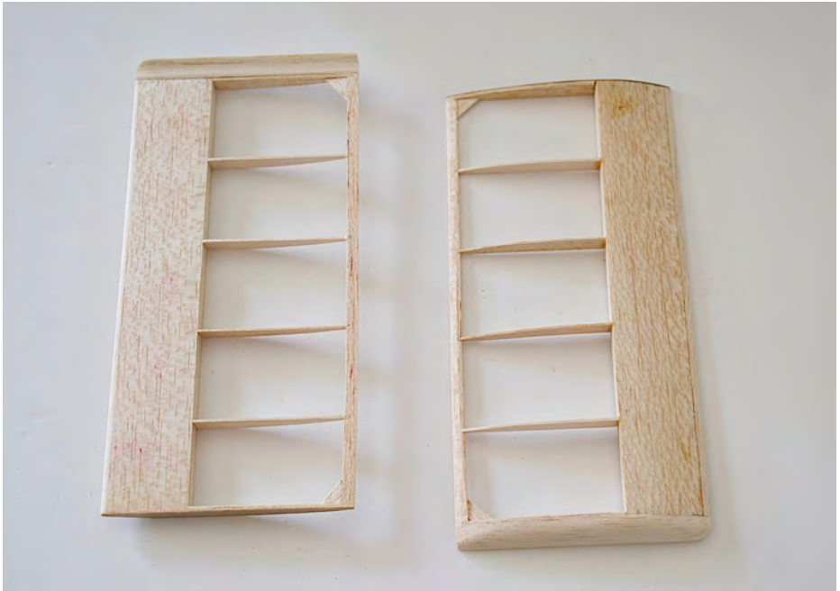
Fuselage progress on Ol' Ironsides showing sheet fuselage sides as in the original and above, D box wing construction.
